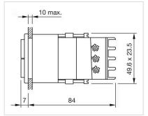
Actuator, 21.2 mm x 41.2 mm, Non illuminated, Rectangular, Black, Plastic, 2 C, Maintained, Screw terminal
