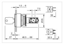
A = Solder terminal B = Plug-in terminal 2.8 x 0.5 mm C = Universal terminal 2.0 mm x 0.5 mm
