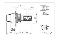
A = Solder terminal B = Plug-in terminal 2.8 x 0.5 mm C = Universal terminal 2.0 mm x 0.5 mm
