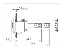
A = Screw terminal B = Plug-in terminal 6.3 mm x 0.8 mm
