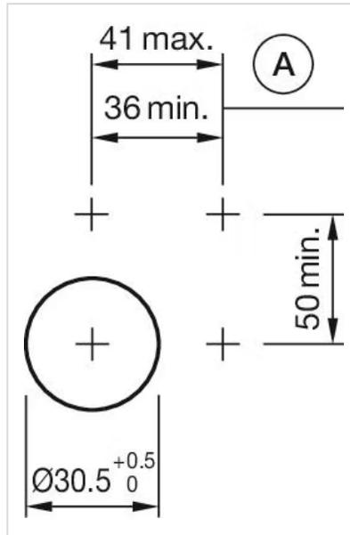
A = Action range of aligning pins
