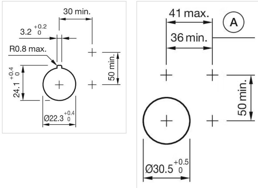
A = Action range of aligning pins
