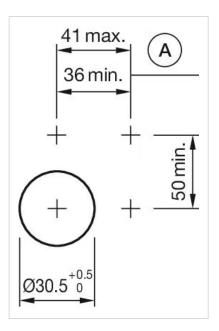
A = Action range of aligning pins
