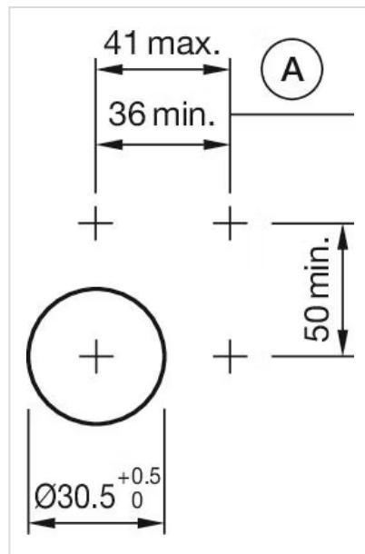
A = Action range of aligning pins
