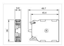
B = Spring-type terminal for Part No. 45-313.1X40
