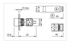
A = Plug-in terminal 2.8 mm x 0.5 mm B = Solder terminal C = Screw terminal
