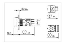
$\label{eq:Absolute} A = \mbox{Plug-in terminal } 2.8 \mbox{ mm x 0.5 mm} \\ C = \mbox{Screw terminal}$
