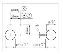
A = Solder/Plug-in terminal 2.8 mm x 0.5 mm B = Solder terminal C = Screw terminal
