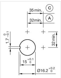
A = Solder/Plug-in terminal 2.8 mm x 0.5 mm C = Screw terminal
