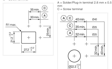
A = Solder/Plug-in terminal 2.8 mm x 0.5 mm
