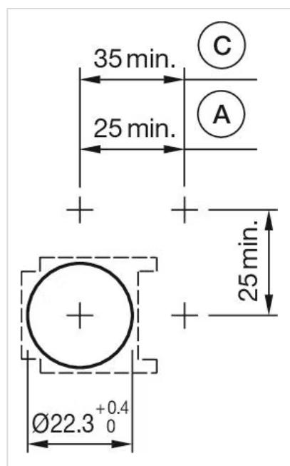
A = Solder/Plug-in terminal 2.8 mm x 0.5 mm
