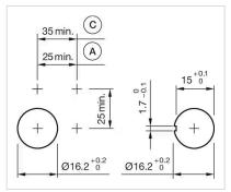
A = Solder/Plug-in terminal 2.8 mm x 0.5
