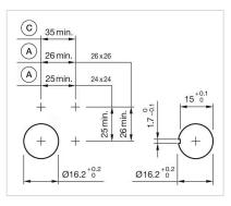
A = Solder/Plug-in terminal 2.8 mm x 0.5 mm
