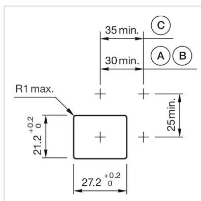
A = Solder/Plug-in terminal 2.8 mm x 0.5 mm
