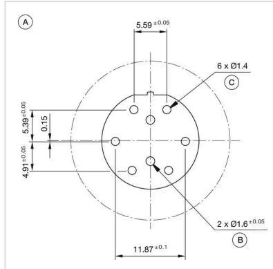
A = Drilling plan (component side)
