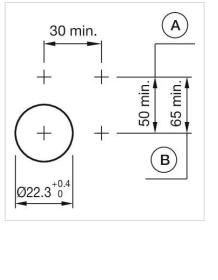
A = Screw terminal B = Push-in terminal (PIT)
