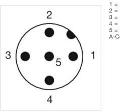
1 = NC 2 = LED+ 3 = Common 4 = LED-5 = NO A-Coded
