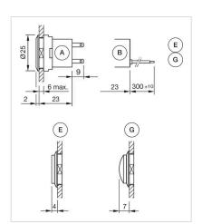
A = Plug-in terminal 2.8 mm x 0.8 mm B = Flat ribbon cable E = Lens raised above bezel
