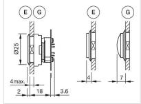
E = Lens raised above bezel G = Lens convexe raised above bezel
