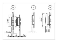
A = Lens level with bezel E = Lens raised above bezel H = Mushroom-head cap
