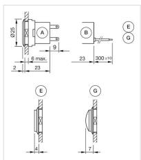
A = Plug-in terminal 2.8 mm x 0.8 mm B = Flat ribbon cable
